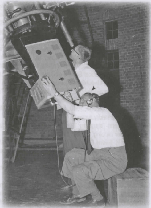
Figure 10. Unidentified operators using image orthicon tube assembly attached to Lamont-Hussey Telescope, 1956. (Lowell Observatory Archives)
